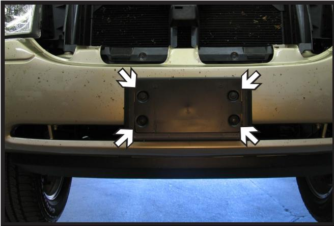
5. If equipped, remove the four (4) push pins from the license plate bracket and set aside.
