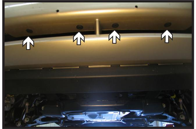
6. On the underside of the lower fascia opening, remove the four (4) push pins. Remove the fascia from the vehicle.
