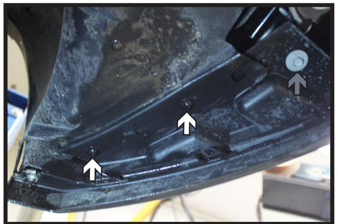
4. On the underside corner of the fascia, using a T20 Torx, remove the two (2) outer screws (white). Then using a 10MM socket, remove the one (1) inner screw (gray). Do this on both sides of the vehicle. Pull the corners of the fascia away from the vehicle disconnecting any electrical connections and set the fascia aside.
