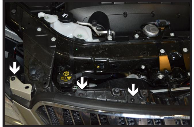
1. Remove the five (5) push pins from the top fascia cover (white). Then pry up the end of the rubber strip, releasing the clip underneath (gray). Do this on both sides of the vehicle. Remove the cover from the vehicle.
