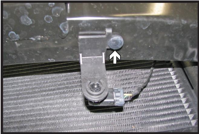
1. Remove the temperature sensor from the bracket, then remove the push pin from the bracket and set the bracket aside.
