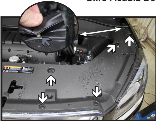
1. Remove the five (5) push pins from the top fascia cover (white). Then pry up the end of the rubber strip, releasing the clip underneath (gray). Do this on both sides of the vehicle. Remove the cover from the vehicle.
