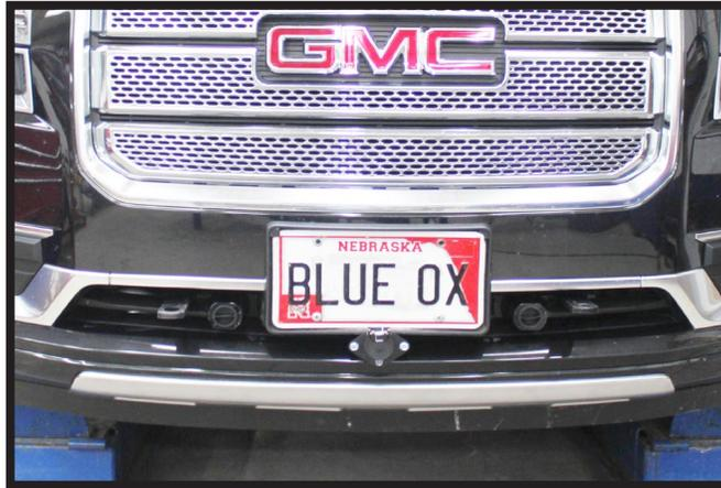
9. Hold the fascia as close to its original position, mark and trim the fascia around the convenience links and attachment tabs. Reinstall the fascia and fascia cover.
