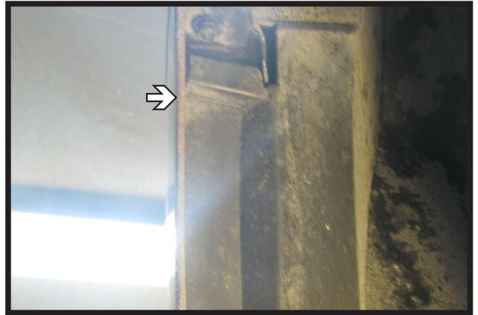
6. Using a 10MM socket, remove the hex bolt holding the horn to the frame rail. Remove the horn and bolt and set aside for later reinstallation. Do this to both sides.
