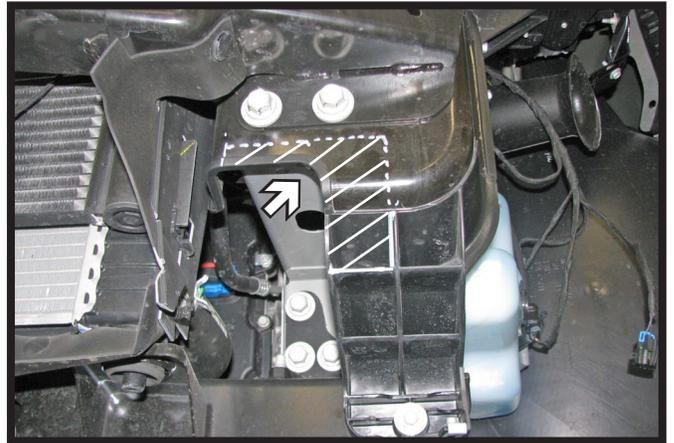
2. Using a reciprocating saw, notch out the shrouding for baseplate clearance. Do this on both sides of the vehicle.
