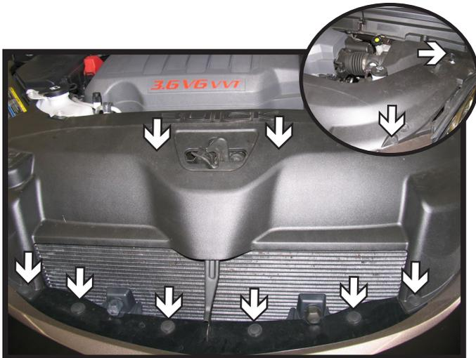
1. Remove twelve (12) push pins from the plastic piece covering the top of the under carriage with a flat screwdriver. There are two (2) push pins on each outer edge of the vehicle (see insert). Also, remove six (6) additional push pins from the bottom segment of the fascia. Remove push pins and set aside for later reinstallation.
