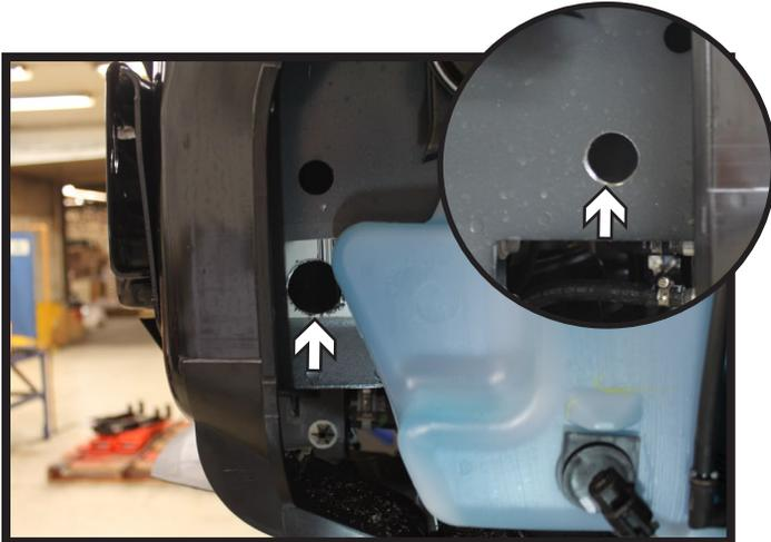
5. Using a 1-1/4" hole saw, drill an access hole into the frame for nut plate installation. Do this on both sides of the vehicle.
