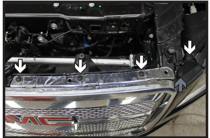
2. Along the top edge of the fascia, using a T20 Torx, remove the four (4) screws from the driver side (white). Then the three (3) on the passenger side. Using a 7MM socket, remove the screw from the edge on both sides of the vehicle (gray).
