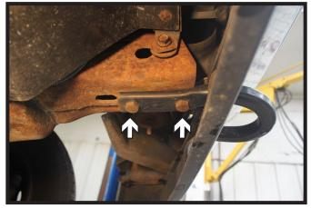
Using a 18MM socket, remove the four (4) bolts from the tow hooks. There are two (2) on each side.
