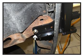
Position the baseplate onto the frame, aligning to the holes in the frame and clamp in place. Install a 1/2"-13 x 1-3/4" bolt with 1/2" lock and flat washers into the rear hole and a 1/2"-13 nut plate on the inside of the frame. Do this on both sides of the vehicle. Fully tighten all hardware.
