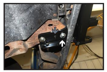
Install a 1/2"-13 x 1-3/4" bolt with 1/2" lock and flat washers into the front hole and a 1/2"-13 whiz nut on the inside of the frame. Do this on both sides of the vehicle. Fully tighten all hardware.
