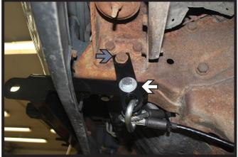
5. Using a 19MM socket, remove the existing bolt from the outside of the frame (gray). Install the safety cable bracket onto the frame, reusing the existing bolt and a 1/2"-13 x 1-3/4" bolt with 1/2" lock and flat washers (white) into the baseplate hole and a 1/2"-13 hex nut on the inside of the baseplate. Do this on both sides of the vehicle. Fully tighten all hardware.
