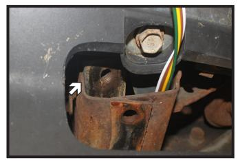
2. Remove the existing nut plates from the tow hook pockets.
