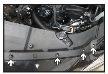
1. Using a T20 Torx, remove the eight (8) screws from the top edge of the fascia. There are four (4) on each side.
