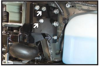
12. Using a 13/32" drill bit, drill the remaining three (3) holes thru the frame. Install 3/8"-16 x 1-3/4" bolts with 3/8" lock washers into the top holes (white) and a 3/8"-16 x 2" bolt with 3/8" lock washer into the lower hole (gray). Secure all bolts with a 3/8" nut plate on the inside of the frame. Fully tighten all hardware. Do this on both sides of the vehicle.
