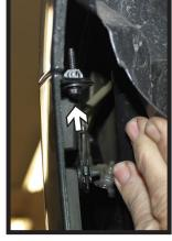
Using a T15 Torx, remove the three (3) screws from wheel well (left). Pull back the wheel well liner and remove the screw at the fascia joint with a 7MM socket (right). Do this on both sides of the vehicle.
