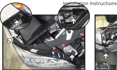
5. Using a 7MM socket, remove the four (4) screws from PS headlight. There are two (2) on the top side, one (1) along the side (left inset) and one (1) underneath (right inset). Disconnect the electrical line and set the headlight aside.
