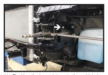
11. Position the baseplate onto the vehicle in between the frame and support plate. Line up the holes of the baseplate and support plate and securely clamp in place.
