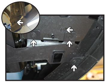
3. Using a 7MM socket, remove the ten (10) screws from the underside of the fascia. There are five (5) on each side.
