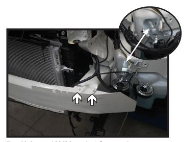
7. Using a 13MM socket & wrench, remove the four (4) bolts from the top edge of the bumper. There are two (2) on each side. Pull the bumper from the vehicle and set aside.
