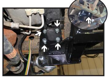
6. Continue drilling the remaining holes in the baseplate thru the frame. Install 1/2"-13 x 1-1/2" bolts with lock washers into the holes and a 1/2" whiz nuts on the inside of the frame. Do this on both sides of the vehicle. Fully tighten all hardware.
