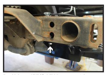
5. Using a 17/32" drill bit, ream out the bottom back hole. Install a 1/2"-13 x 1-1/2" bolt with lock washer into the hole and a 1/2" whiz nut on the inside of the frame. Do this on both sides of the vehicle. Fully tighten all hardware.
