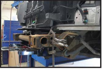
4. Position the baseplate onto the frame, lining up front hole on the underside of the frame and the back hole of the baseplate. Square and clamp the baseplate securely to the frame.
