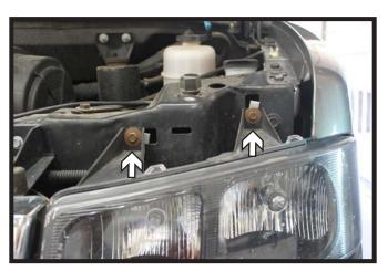
Using a 10MM socket, remove the two (2) screws from the headlight. Disconnect all electrical connections and set aside. Do this on both sides of the vehicle.
