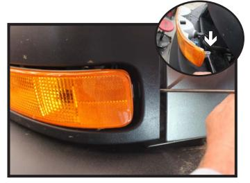
Using a flat screwdriver, pry behind the grille to release the clip and release the park light from frame. Disconnect all electrical connections and set aside. Do this on both sides of the vehicle.
