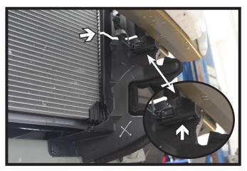
8. On the driver side, remove the temperature sensor from the shrouding (inset). Then trim off the lower section of the shrouding flush with the bottom of the bumper.
