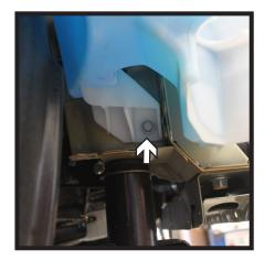
On the passenger side, remove the push pin from the washer reservoir just below the blinker (left). Using a 10MM socket, remove the upper screw (middle) and lower screw (right) from washer reservoir. Disconnect all lines and set reservoir aside.
