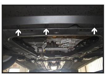
5. Remove the three (3) push pins from the underside of the fascia towards the center. Gently pry the fascia from the vehicle, disconnecting any electrical connections and set the fascia aside.
