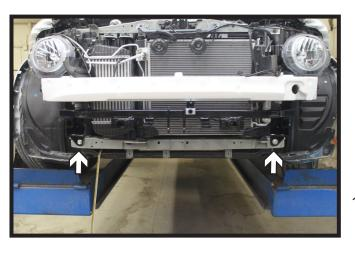
13. Using a 1/2" drill bit, ream out the two(2) top existing holes for bolt clearance (white).
