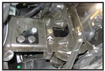
Slide baseplate into place. Insert one (1) 5/8" x 3-1/2" bolt into the existing hole. Tighten fully. Do this on both sides of the vehicle.
