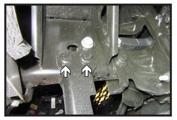
Using a 24MM socket, remove the two (2) bolts from the bracket. Remove tow hook and bracket, set aside, it will not be reinstalled. Do this on both sides of the vehicle.
