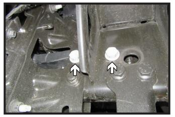
1. Using a 24MM socket, remove the two (2) bolts from the tow hook. Do this on both sides of the vehicle.
