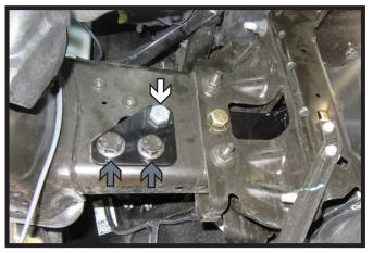
Place spacer brackets on both sides of the frame as shown. Install one (1) 5/8" x 4-1/2" bolt (white). Then install the two (2) existing 16MM bolts (gray). Tighten all bolts fully. Do this on both sides of the vehicle.
