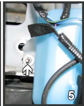
4. On the driver's side, using an 8MM socket, remove the bolt holding the horn. Set the horn and bolt down by the side to be reinstalled later.
