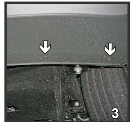
3. **MKT models:** In front underneath, remove three push pins from the center. Using a 5.5MM socket, remove one bolt on each side (gray arrow). Pull fascia corners out to the side of the vehicle to unsnap, then pull forward. Set fascia, pins and bolts aside carefully to be reinstalled later.
