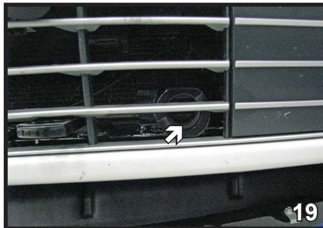
19. Hold the fascia up in front of the baseplate, mark and trim the area needed for the baseplate to come through. The installation of the baseplate is complete.
