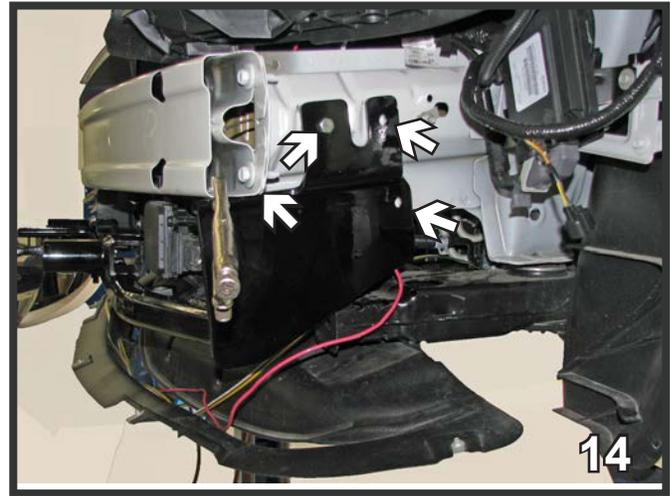
13. First using the baseplate as a template with a 13/32" drill bit, drill two holes underneath. Insert a 3/8"-16 x 2 1/2" bolt into the holes with 3/8" lock washers and 3/8"-16 nut plate, tighten with Loctite Red. Do the same on both sides of the vehicle.
