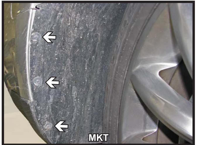
2. **MKS** models: Using a phillips screwdriver, remove the four (4) screws that are located just forward of the front tire on both sides of the vehicle. Set screws aside to be reinstalled later.
