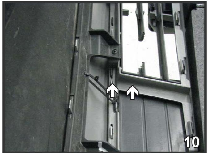
9. **MKS models:** On the back side of the fascia by the cruise control mechanism, using a utility knife, trim across the bottom, as shown. Do this to both sides of vehicle.
