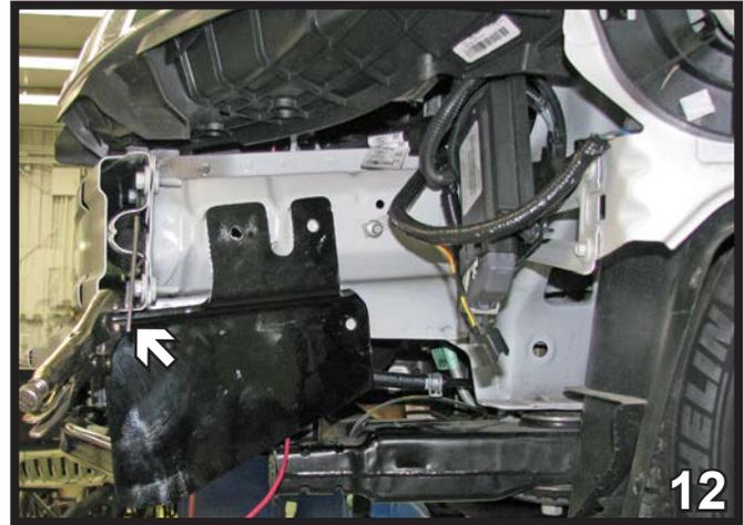
11. **MKS models:** Underneath the vehicle, using a flat screwdriver, remove seven push pins. Set the plastic cover and push pins aside to be reinstalled later.
