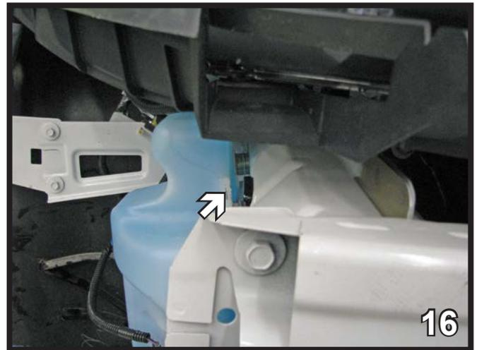
15. On the passenger side before reinstalling the washer reservoir, using a utility knife cut off the top right installation tab about 1 1/2" x 1 1/2". Be careful not to cut into reservoir. Reinstall the water tank and connect the hoses and plug in electrical connections.
