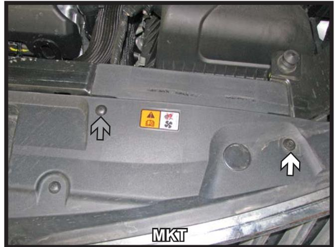
1. **MKS** models: Using a 10MM socket, remove the two (2) bolts (white arrows) from the top of the fascia on both sides of the vehicle. Use a flat screwdriver to remove the push pin in the center (grey arrow). Set bolts and push pins aside to be reinstalled later.
