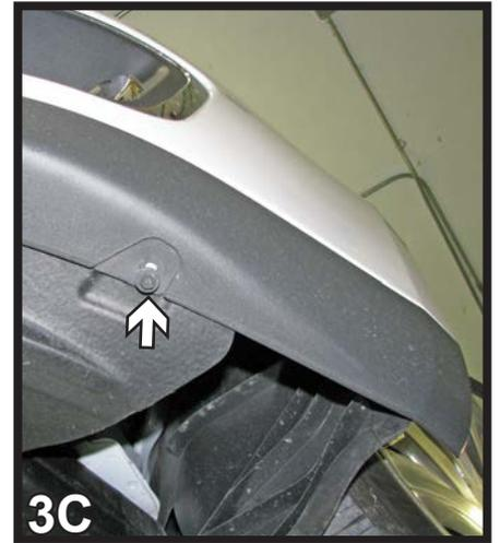
3. **MKS models:** On the underside use an 8MM socket to remove the bolts (white arrows). There is one (1) bolt on the outermost edges of the fascia, figure 3C, one (1) directly in the center, figure 3A, and also one (1) between the push pins, figure 3B.
