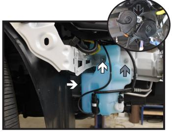
4. Using a 11MM socket, remove the two (2) screws from the inner edge of the washer fluid reservoir (white). Then using an 8MM socket, remove the outer screw (gray). Disconnect all lines and set reservoir aside.
