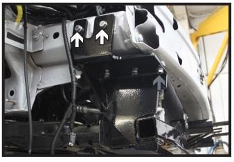
8. Using a 3/8" drill bit, drill the remaining three (3) holes thru the frame and bumper. Install two (2) 3/8"-16 x 1-1/4" bolts and 3/8"-16 nut plates into the top holes (white). In the lower bumper hole, install a 3/8-16 x 2" bolt with 3/8"-16 nut with 3/8" washers in between the bumper & baseplate as a spacer (gray). Do this on both sides of the vehicle. Tighten all fasteners.
