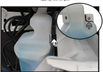
9. Mark and trim the front tab of the washer fluid reservoir (gray). Reinstall the reservoir, using the supplied 1/4" washers as a spacer on the top rear hole (white).
