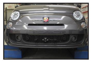
10. Hold the fascia up to the vehicle as close to it's original position. Mark and trim with a utility knife until the fascia is clear of the attachment tabs and convenience links. Reinstall the fascia.
