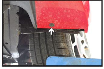
Using a phillips screwdriver, remove the one (1) screw from the underside bottom corner of the fascia. Repeat on the other side of the vehicle.
