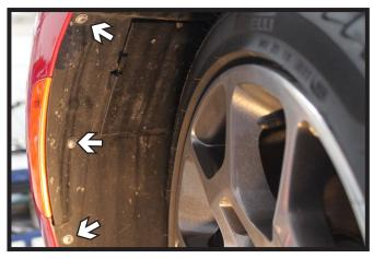
Using a phillips screwdriver, remove the three (3) screws from the wheel well in front of the tire. Repeat on the other side of the vehicle.
