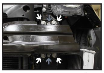
7. Using a 15MM socket, remove the four (4) larger bolts from bumper (white). Then using a 10MM socket, remove the two (2) smaller bolts (gray). Repeat on the other side of the vehicle. The metal bumper and smaller bolts will not be reused.
