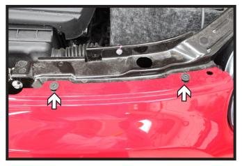
Using a T30 Torx, remove the four (4) screws from the top edge of the fascia. There are two (2) on each side.
