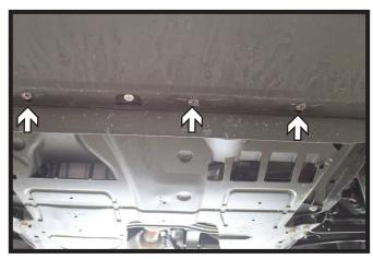
Using a T30 Torx, remove the three (3) screws from the underside of the fascia. DO NOT remove the silver screw.
