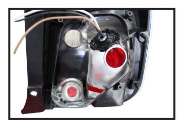
11. Possible location for the BX8869: Using a 20 Torx remove the four (4) screws from the back plate and remove (Right). Using a 1" hole saw drill a hole into the metal portion of the light as shown. Put the wires thru and silicone around the hole to seal.
