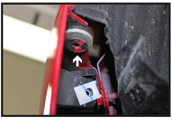
Using a T30 Torx, remove the screw from behind the wheel well cover where the fascia meets the fender. Repeat on the other side of the vehicle.
