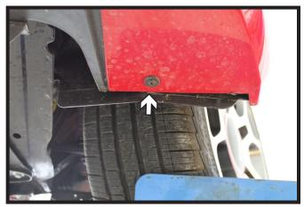
Using a Phillips screwdriver, remove one
