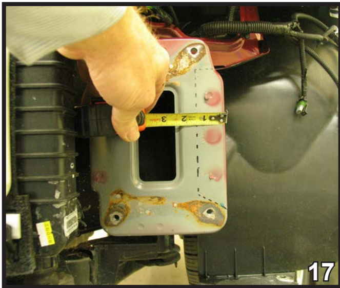
17. Measure and mark on the side of frame end 1-1/2" wide. Do this to both sides. **NOTE: 1-1/2" measurement may vary depending on the model of vehicle and is intended to be flush with side of the frame (see photo in Step 19).
