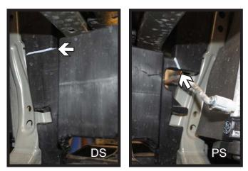
3. **iM models only:** Trim the plastic shielding under the bumper and remove the lower section.
