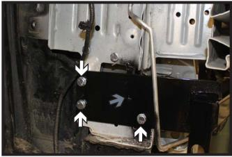
Using a 3/8" drill bit, drill the remaining holes in the sideplates thru the frame. Install the 3/8" hardware into the holes. Do this on both sides of the vehicle. Fully tighten all hardware.
