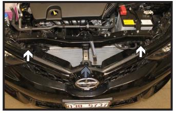
Remove the two (2) push pins from the fascia (white). Then, using a 10MM socket, remove the screw from the center of the fascia (gray).
