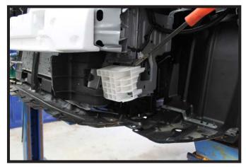
2. **tC models only:** On the driver side, remove the plastic reinforcement and set aside. The reinforcement will not be reinstalled.
