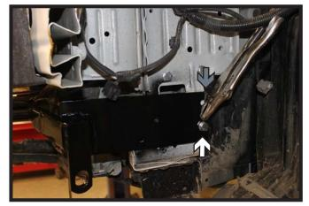
Install the baseplate onto the frame, flushing the edge of the sideplate with the frame (gray) and clamp in position. Using a 3/8" drill bit, drill the lower back hole (white) thru the frame. Install the 3/8" hardware into the hole. Do this on both sides of the vehicle. Fully tighten all hardware.
