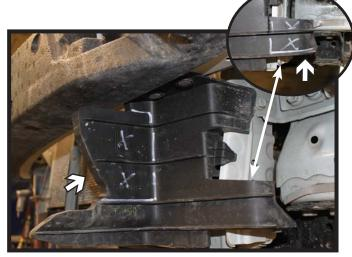
3. **tC models only:** On the driver side, trim the plastic shielding under the bumper and towards the outer edge as shown for baseplate clearance.
