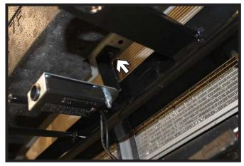
13. **Optional Breakaway:** Attach the bracket to the lip of the bumper at the desired location with the #12 screw provided. Attach the breakaway to the bracket with the 1/4" hardware provided.
