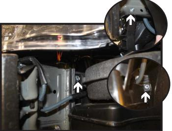
2. **iM models only:** On the driver side, using a 10MM socket, remove the three (3) screws from the baffle. There is one (1) in front under the headlight and two (2) just in front of the wheel well liner (insets). Set the baffle aside.
