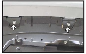
4. Using a 10MM socket, remove the eight (8) screws from the underside of the fascia. There are two (2) on each side and four (4) along the front.
