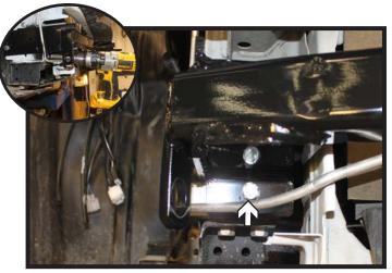
Using a 3/8" drill bit, drill the front hole thru the frame. Install the 3/8" hardware into the hole. Do this on both sides of the vehicle. Fully tighten all hardware.
