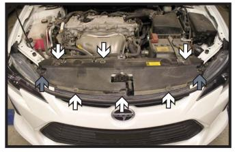
Push down on to release and remove the six (6) push pins from the fascia cover (white). Then remove the two (2) bumpers (gray) and set the cover aside.
