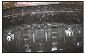
3. Using a 10MM socket, remove the six (6) screws from the underside of the fascia. There are two (2) on each side and four (4) along the front.
