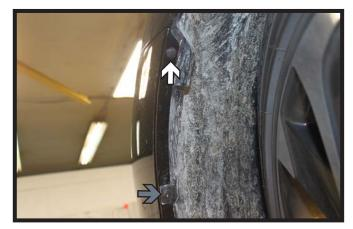
2. Remove the push pin from the edge of the wheel well (white). Then turn the locking pin (gray) to release the fascia from the wheel well liner. Do this on both sides of the vehicle.
