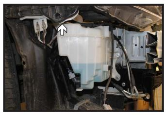
Reinstall the washer reservoir with the spacers, 6MM & 1/4" hardware provided. Note: The upper back bolt will not be reinstalled due to the use of the spacers **iM models only:** Reinstall the baffle on the driver side.
