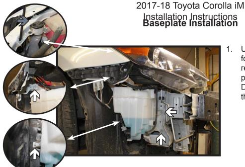
Using a 10MM socket, remove the four (4) screws from the washer reservoir (white). Remove the push pin from the reservoir neck (gray). Disconnect/plug all lines and set the reservoir aside.
