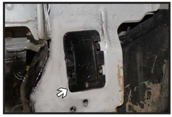
5. **tC models only:** On the driver side, remove the plastic cover along the side of the frame.
