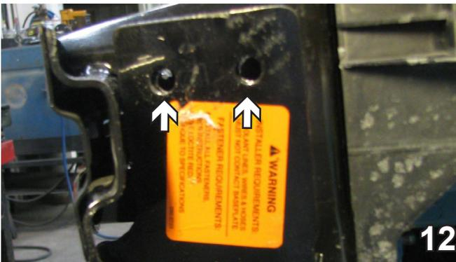
12. Using the baseplate as a template, drill two (2) holes on the side. Do this on both sides using a 13/32" drill bit.
