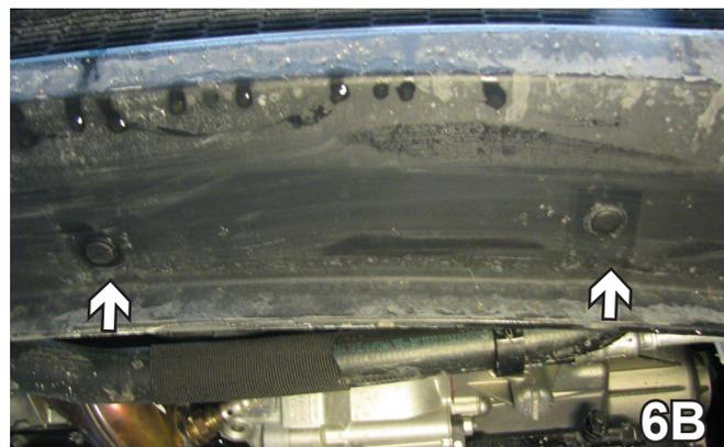
5. There is also a torx 25T bolt (photo 6A) to be removed from both sides using a torx wrench. Remove the three (3) push pins in the center (photo 6B). Pull the fascia forward, disconnect side running and fog lights. Set aside carefully for later reinstallation.
