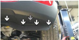
5. Remove four pushpins from the edge of the bottom of the fascia on both sides. There is also a torques 25T bolt (gray arrow) to be removed from both sides using a torques wrench. There are three other pushpins in the center, remove them. Eyebolts need to be removed from the fascia to remove the fascia. Pull the fascia forward, disconnect side running and fog lights. Set aside for later reinstallation.
