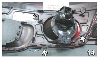
14. The wire air sensor needs to be moved behind the fog light. It originally was placed around the top of the fog light (gray arrows) and needs to be placed and taped below the fog light. Cut off a clip and tape to the sensor below the fog light.
