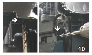
Using the baseplate as a template, drill two holes underneath the baseplate and two holes on the side. Do this to both sides using a 13/32" drill bit.
