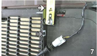
7. Located on both sides behind the grill, there is a temperature sensor that will need to be moved. Trim 1 1/8" from the top to remove the notch holding the sensor, cut and remove the webbing with it, and replace the sensor in another notch we will cut out a little further down (gray arrow).
