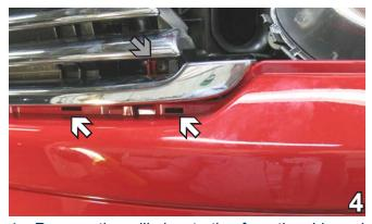
4. Remove the grille by starting from the side and releasing the clips. They will fit back in when reinstallation occurs. By the wheel well there is a bolt that needs to be removed with a 10MM socket. Also, after removing the grille, there are two bolts that need to be removed with a 10MM socket. (gray arrow) Do to both sides and set aside for later reinstallation.
