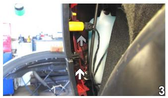
3. After removing the wheel well cover, remove one pushpin connecting the fascia using a flat screwdriver. Also remove the small yellow light (gray arrow). Do this to both sides. Set pushpins aside for later reinstallation.
