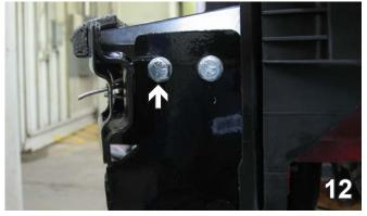
Into the holes drilled in the side also insert 3/8-16 x 1 1/4" bolts with Loctite, 3/8" lock washers and 3/8" nut plates. Do this on both sides.
