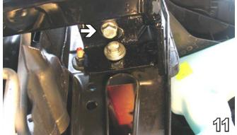
11. Insert 3/8-16 x 1 1/4" bolts with Loctite, 3/8" lock washers and 3/8" nut plates into the drilled holes on the bottom. Do this on both sides.
