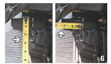
6. You will need to cut the air dams 3" down and 2.5" in to make room for the baseplate. Do this to both sides. These will not be reinstalled.
