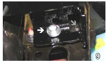
9. Trim the threads off the outer bolt flush with the nut (gray). Do this on both sides of the vehicle.
