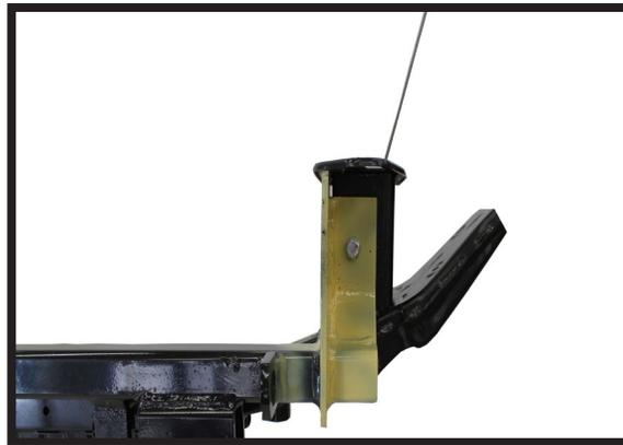
11. Place baseplate onto bumper frame. The back edge of the baseplate should be flush with the bumper frame bracket. Using a 13/32" drill bit and the baseplate as a template, drill out the holes. Do this on both sides.
