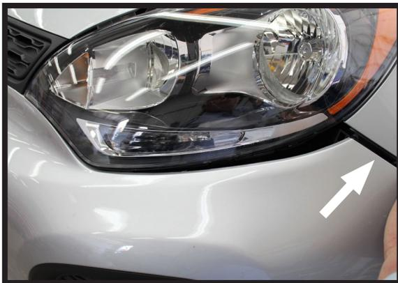
5. Pull the front fascia away from the front of the vehicle. Gently pry the fascia away from under the headlight area.
