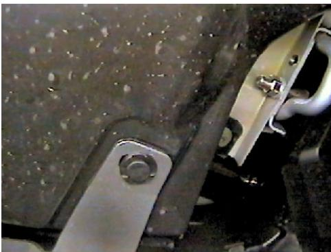
5. Remove push pin from tab on lower edge of fascia, both sides.
