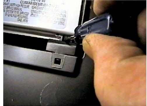
2. Using a small flat screw driver, push the four tabs down between the top edge of fascia and upper cross member while pulling fascia forward to release from cross member.
