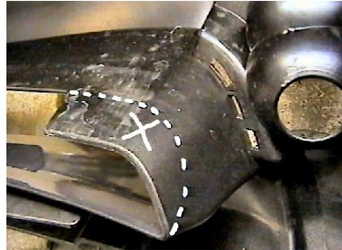
19. Set fascia face down on a soft material to prevent scratching, mark and cut back side of fascia just between fog lights top of opening, as shown in photo, using the utility knife. Reinstall head light assemblies, metal bumper and fascia. **Be sure all electrical components are plugged in properly.**
