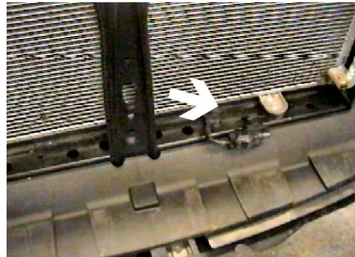
16. Bend temperature bracket and sensor back toward radiator. It may be necessary to bend bracket more when base plate is installed and may differ from vehicle to vehicle.
