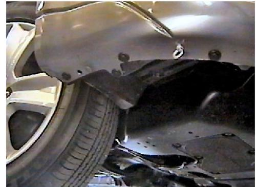
4. Forward of front tires are four push pins to remove from lower edge of fascia, both sides.
