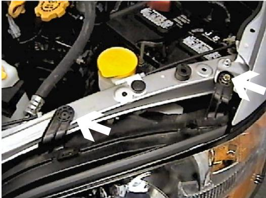
7. Using the 10MM socket, remove metric bolt from head light assembly and one push pin, both sides.
