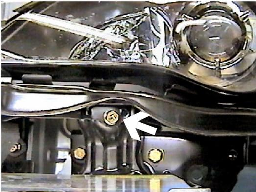
9. Remove metric bolt from front of head light assembly with the 10MM socket, both sides.
