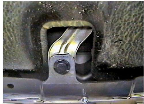
6. Remove push pin from tab on lower center edge of fascia.
