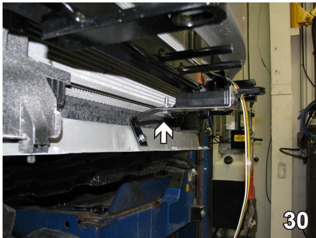
30. Attach the breakaway to the bracket with a 1/4"-20 x 3/4" hex bolt, 1/4" lock washer and 1/4"-20 hex nut.
