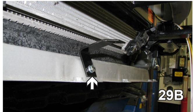
29. Using the hole in the middle of the lower frame. Attach the breakaway bracket with a 6MM-1 x 16MM hex bolt and a 1/4" lock washer inserted into the hole.
