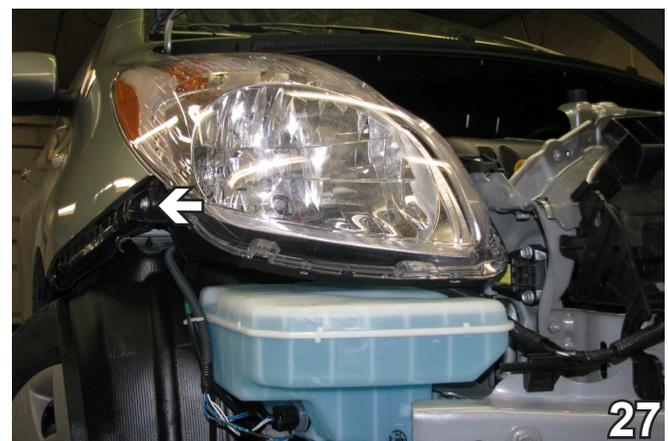
27. Reinstall the headlight. Reconnect all electrical connections and clamps.
