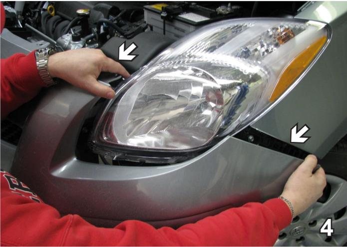
4. Pull fascia corners out to the side of the vehicle on both sides, then forward. Set fascia aside carefully for later reinstallation.
