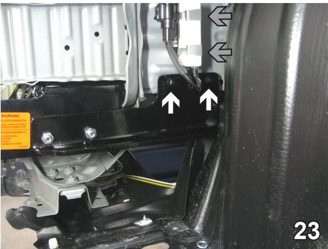
23. Temporarily bolt tight the lower bracket to the baseplate with just 3/8"-16 x 1" bolts and 3/8" hex nuts only. Align the back of the bracket holes to the center of the lower frame webbing. Use as a template to drill the back two holes with a 13/32" drill bit (white arrows). Do this on both sides. On the driver's side only, use a 10MM socket to remove the bolts (gray arrows) holding the sensor so that it can be set out of the way while drilling then replace.
