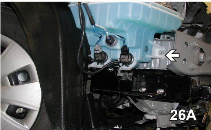
26. **2007-11 Models (28A):** On the passenger side, reinstall the washer reservoir. Reconnect the electrical connections and the hoses.
