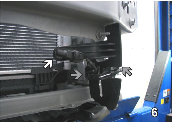
6. On the driver's side, remove the temperature sensor (white arrow). Unhook the plastic guard under the bumper (gray arrow) on both sides and set aside. Set sensor aside for later reinstallation.
