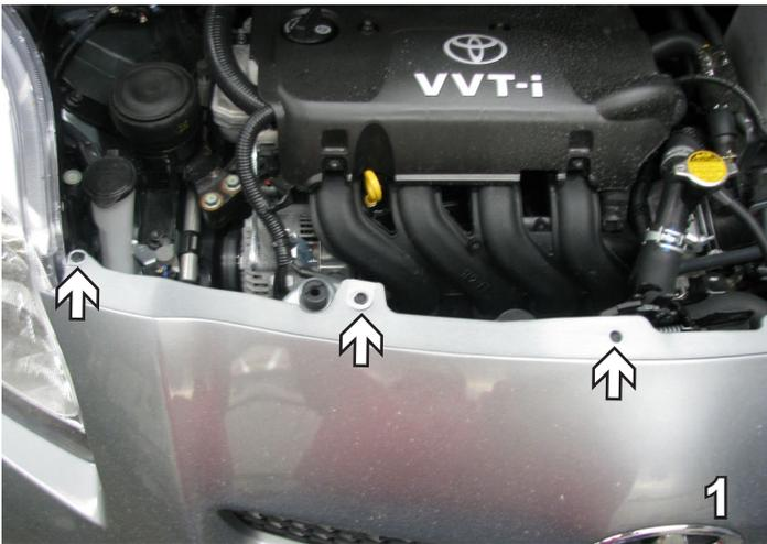
1. Push in center to remove plastic push pins from top edge of fascia. Set push pins aside to be reinstalled later.
