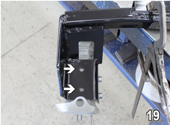
19. Using the baseplate as a template, drill the two bottom holes with a 13/32" drill bit into the frame extension. Install 3/8"-16 x 1-1/4" bolts and 3/8" lock washers into drilled holes. Then tighten into 3/8" nut plates inside the extension. Use Loctite Red on all bolts. Do this to both sides.
