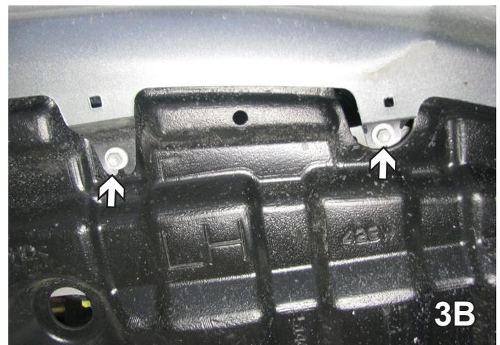
3. Remove eight (8) metric bolts from lower edge of fascia all the way around using a 10MM socket. Set bolts aside for later reinstallation.
