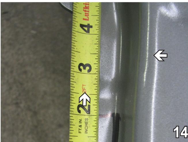
14. Measure up 2" on the edge of the bumper core. Use a reciprocating saw to cut flush with the bumper. Do this on both sides.
