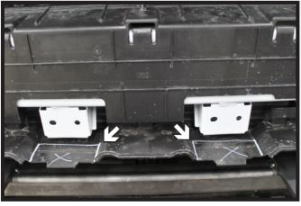
Using a utility knife, trim two (2) pockets in the plastic shrouding back flush to the metal brackets as shown.
