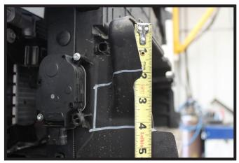
7. Trim the radiator shrouding approximately as shown for baseplate clearance. Do this on three (3) shrouds across the front of the vehicle.
