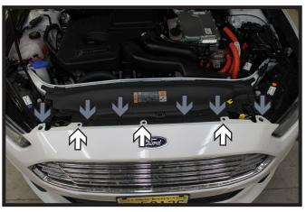
1. Using a T25 Torx, remove the three (3) screws from the top edge of the fascia (white). Remove the six (6) push pins from the top edge of the fascia (gray).
