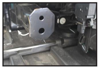
9. Using a hammer, knock the edge of the extension behind for baseplate clearance. Do this on both sides of the vehicle.
