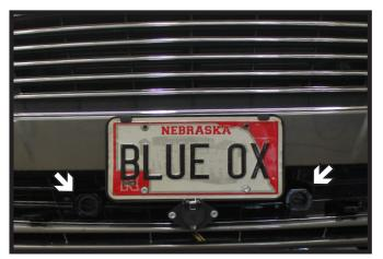
14. Hold the fascia as close to its original position, mark and trim the fascia around the convenience links and attachment tabs. Make sure to only trim as little as necessary to allow for tabs. The ACC unit on the driver side may malfunction if too much plastic is cut away. Important: Ensure that nothing is installed in front of the ACC sensor. Obstructions will cause false readings from the sensor. Reinstall the fascia.
