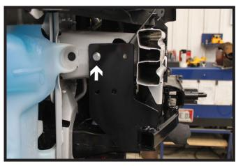
10. Using the existing hole, bolt the baseplate to the frame with a 3/8"-16 x 1" bolt, 3/8" lock washer and 3/8"-16 nut plate. Do this on both sides of the vehicle. Level and tighten down the baseplate.
