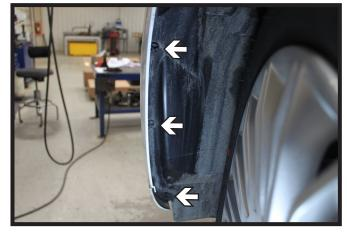
Remove the three (3) push pins from the outer edge of the wheel well. Do this on both sides of the vehicle.
