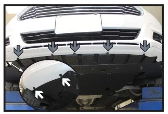
3. Using a 7MM socket, remove the five (5) screws from the underside edge of the fascia (gray). Remove the push pins from the underside corners, there are two (2) on each side (white).
