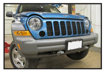
14. Reinstall fascia and grill. Replace the plastic rivets provided that were remove in step 5. Be sure that all electrical components are plugged in properly.
