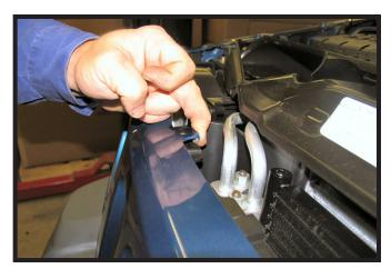
Lift the two (2) tabs on the top edge of grill between headlights and pull grill center forward to release tabs.
