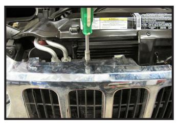
Using the T20 Torx, remove the two (2) bolts from the top edge of grill.
