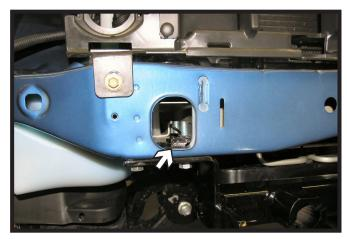
11. Align baseplate with the two (2) existing holes in the bottom of frame, insert backing plate and nut plates into opening on the end of frame rail to align with these existing holes. Do this on both sides of the vehicle. Some vehicles may need to have these existing holes reamed to acquire proper fit. Tighten the 3/8" hex bolts, flat and lock washers with the 9/16" socket. Do this on both sides of the vehicle.
