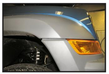
8. Release tab on the inside of wheel well and pull fascia corner to the side. Do this on both sides of the vehicle.
