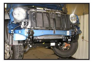
13. Reinstall hubs on the front of metal bumper using the existing bolts. Attach the permanent baseplate safety cables to the provided convenience link on the baseplate. Additional options may interfere with suggested mounting; in this case, secure the cables to a solid piece of the frame as described in the General Information sheet. Be sure the safety cables do not rub against any hoses or moving parts. Do this on **BOTH** sides of the vehicle.
