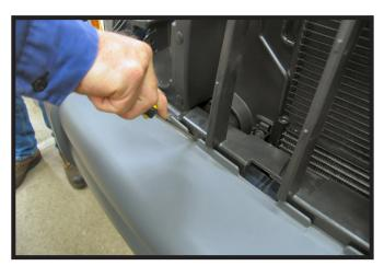
Push the two (2) tabs down with the flat screw driver, pull fascia forward, unplug electrical connections, if applicable and set aside to be reinstalled later.
