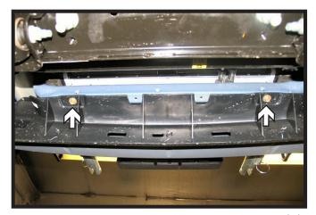
Using a 10MM socket, remove the two (2) bolts from the bottom edge of fascia just below radiator support.
