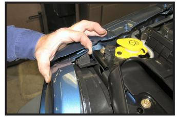
Lift tab just above headlight assembly and pull that portion of the grill forward to release tab. Do this on both sides of the vehicle.
