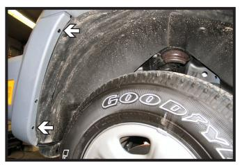
Remove the two (2) push pins from the wheel well edge. Do this on both sides of the vehicle.
