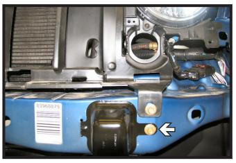
Using a 10MM socket, remove the one (1) bolt from hub. Do this on both sides of the vehicle. Remove hub and set aside to be reinstalled later.
