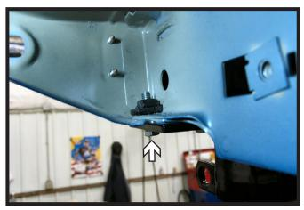
12. Using a 13/32" drill bit, drill a hole into the frame using the baseplate at a template Insert nut plate into opening on the back side of frame support to align with drilled hole. Install the 3/8" hex head bolt and lock washer. Do this on both sides of the vehicle.
