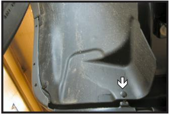
Remove push pin from lower edge of wheel well just forward of the front tire. Do this on both sides of the vehicle.
