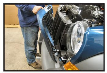
4. Pull the top of grill forward and up, set grill aside to be reinstall later. Using a 10MM socket, remove the one (1) bolt just below the headlight assembly. Do this on both sides of the vehicle.
