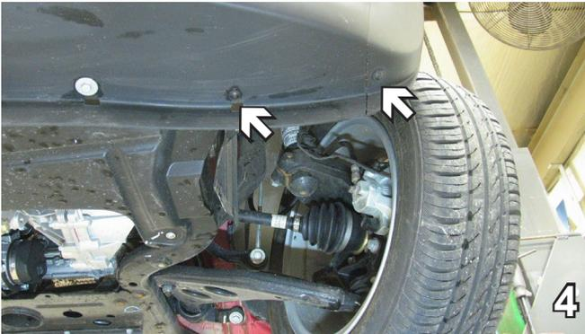
4. Remove the two Phillips screws from the lower edge of front fascia, on both sides.
