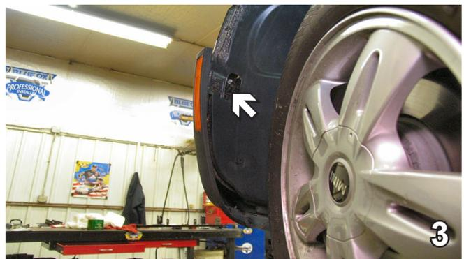
3. Locate opening in wheel well just forward of front tire, remove two metric bolts with the 8MM socket, on both sides.
