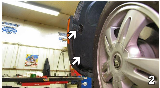
2. Just forward of front tire, on wheel well, are two Phillips head push pins to remove, on both sides.
