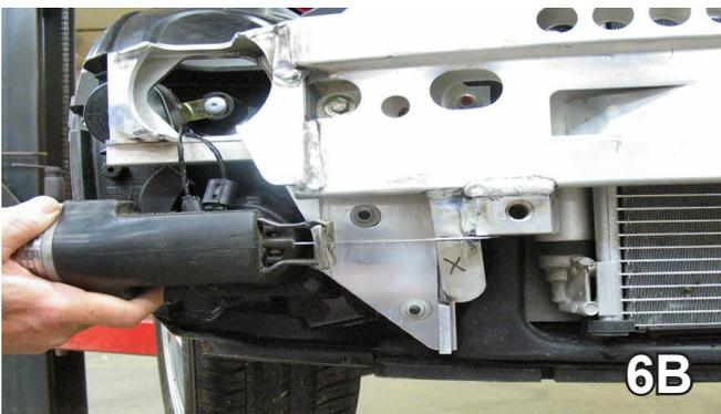
6. Locate tow plate bracket on passenger's side of front bumper. Mark and remove lower gusset just below tow plate bracket with the reciprocating saw, as shown in photos above. This will open area to allow baseplate installation.
