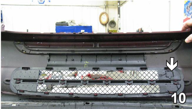
10. Hold fascia as close to its original location as possible on the vehicle. Mark and trim lower grill around the convenience links and attachment tabs. Reinstall fascia. **Be sure all electrical components are plugged in properly.**
