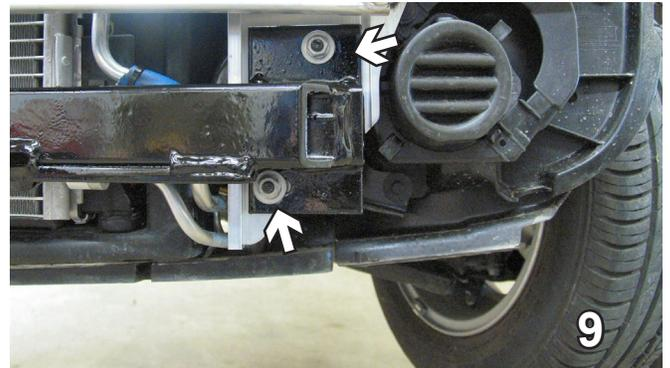
9. Align holes of baseplate with studs just below metal bumper and reinstall four existing nuts. **Be sure and use loctite on all threads before tightening. Tighten all nuts 16 ft/lbs.**
