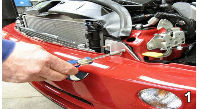
1. Using the T30 Torx, remove the bolts from the top side of fascia.
