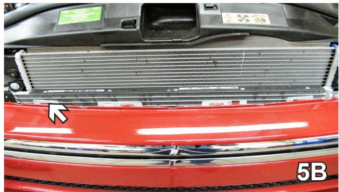
5. Remove three metric bolts from the lower edge of front fascia with the 10MM Socket. Release the four clips on the top edge of fascia, pull fascia forward, unplug all electrical connections and set fascia aside carefully.
