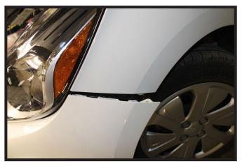
5. Pull the corners of the fascia away from the vehicle disconnecting any electrical connections and set the fascia aside.
