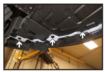
4. Using a 7MM socket, remove the eight (4) screws from the underside of the fascia. There are three (3) on each side and two (2) in the center.
