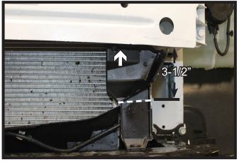
6. Measure down approximately 3-1/2" and cut thru the plastic shielding. Remove the upper push pin and discard the upper portion of the shielding. Do this on both sides of the vehicle.
