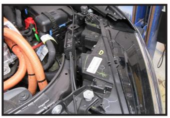
7. Using a T25 Torx, remove the one (1) screw from the headlight. Using a 10MM socket, remove the two (2) bolts holding the headlight in. Slide the headlight out. Do this for both sides of the vehicle.
