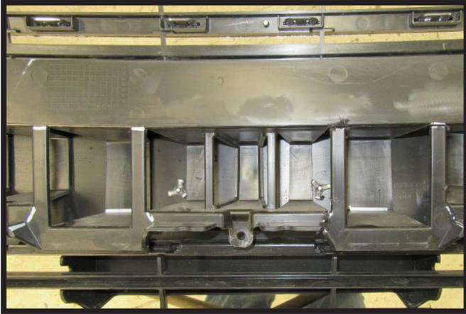
16. On the back side of the fascia use the reciprocating saw to remove the pieces as marked on both sides near the center of the fascia.
