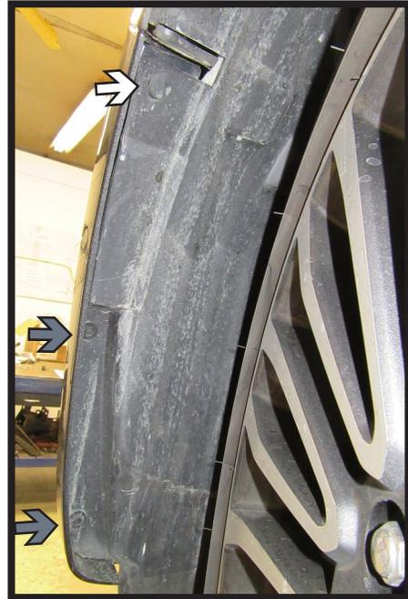
2. In front of the tire, in the wheel well, remove one (1) push pin (white). Using an 8MM socket, remove two (2) bolts (gray). Do this for both sides of the vehicle.
