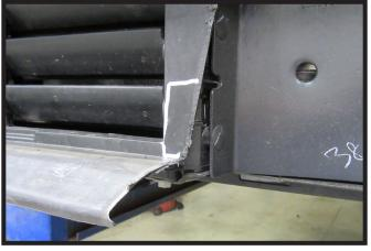
13. Using a recipricating saw notch and remove marked area right under the gusset to the corner and then down. Do this only on the driver's side of the vehicle.
