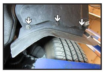
4a. Remove the belly pan. Using a 7MM socket remove the three (3) bolts in front of the tire on both sides of the vehicle.
