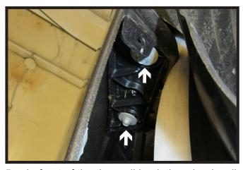
5. In front of the tire, pull back the wheel well cover. Using an 10MM socket, remove the two (2) revealed bolts. Do this for both sides of the vehicle.
