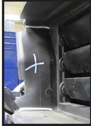
12. Using a recipricating saw remove the marked areas on both sides of the vehicle next to the shutters.
