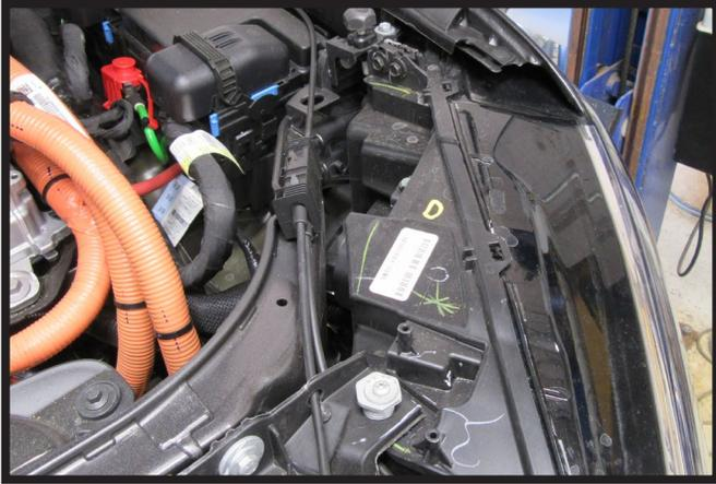
7. Using a T25 Torx, remove the one (1) screw from the headlight. Using a 10MM socket, remove the two (2) bolts holding the headlight in. Slide the headlight out. Do this for both sides of the vehicle.
