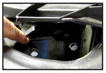
18. Slide the baseplate Into position and insure it is level and aligned with existing holes, before clamping to the frame rail on both sides with large vise grips. Insert 3/8"-16 x 1-1/2" Hex Head Bolt with 3/8" lock washer into the top two (2) pre-existing holes on both sides of the vehicle, with the 3/8" nut plate on the inside of the frame.
