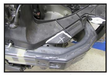
9. Using a reciprocating saw, trim the plastic shrouding approximately as shown for baseplate clearance.
