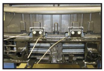
21. Using the baseplate as a template run a 3/8" drill bit through each of the four (4) holes at the top of the baseplate. Then insert the 3/8" nut plate and 3/8" x 1-1/4" lock washer.
