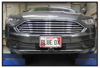
22. Hold the fascia as close to its original position, mark and trim the fascia around the convenience links and attachment tabs. Make sure to only trim as little as necessary to allow for tabs. The ACC unit on the driver side may malfunction if too much plastic is cut away. Important: Ensure that nothing is installed in front of the ACC sensor. Obstructions will cause false readings from the sensor. Reinstall the headlights, fascia, and fascia cover.
