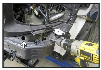
10. Using a 1-1/4" hole saw, drill access holes in the side of the frame on both sides of the vehicle as shown (white).
