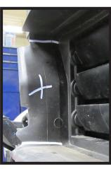
12. Using a recipricating saw remove the marked areas on both sides of the vehicle next to the shutters.
