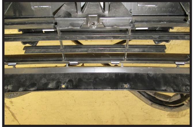
17. On the back side of the fascia near the bottom use a reciprocating saw to trim the four (4) tabs so that they are flush with the rest of the fascia.
