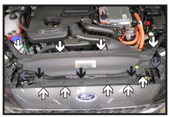
1. Remove nine (9) push pins (white) from the fascia cover. Remove fascia cover and set aside. Using a 10MM socket, remove three (3) bolts (black) from the top of the fascia, and two (2) bolts (gray) from the plastic covers.
