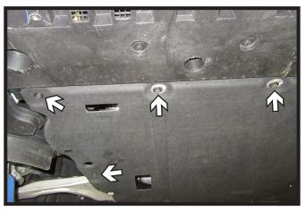
4b. Then using a 10MM socket remove the eight (8) bolts along the middle, four (4) on each side.
