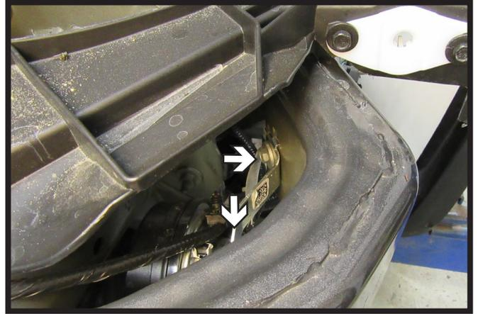
8. Using a 10MM socket, remove the two (2) bolts holding the horn bracket in place. Remove the horn bracket. Do this for both sides of the vehicle.
