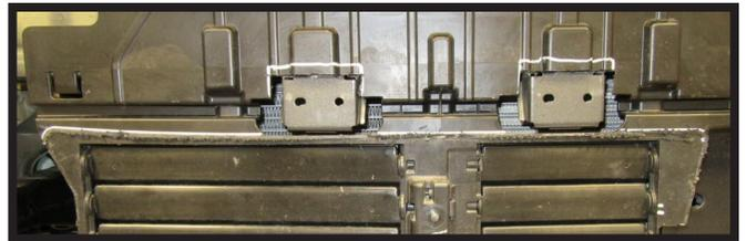
15. Using a recipricating saw remove the marked areas above the shutters. (The top picture is the before and the bottom picture is the after.)
