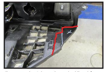
11. Using a reciprocating saw, trim the plastic shrouding approximately as shown (red lines) for baseplate clearance.
