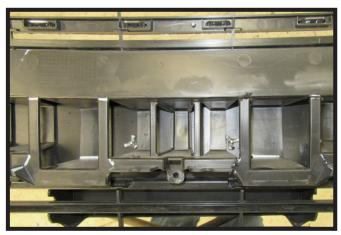
16. On the back side of the fascia use the recipricating saw to remove the pieces as marked on both sides near the center of the fascia.
