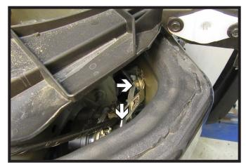
8. Using a 10MM socket, remove the two (2) bolts holding the horn bracket in place.
