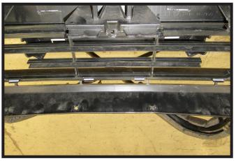
17. On the back side of the fascia near the bottom use a recipricating was to trim the four (4) tabs so that they are flush with the rest of the fascia.
