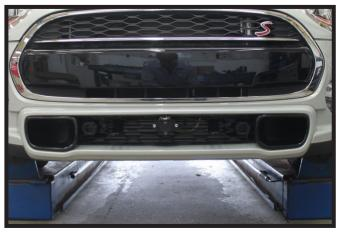
18. Hold the fascia as close to its original position, mark and trim the fascia around the convenience links and attachment tabs. Reinstall the washer reservoir and fascia.
