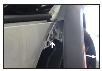
4. Pry the fender flare away from vehicle. Using a T30 Torx, remove the screw from behind the fender flare. Do this on both sides of the vehicle.
