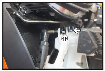
Using a T30 Torx, remove the two (2) screws from the washer reservoir.
