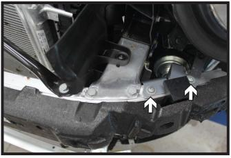
6. On the driver side, using a T30 Torx, remove the two (2) screws from the horn bracket. Disconnect all lines and set the horn assembly aside.
