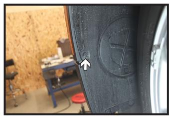
Using a 8MM socket, remove the screw from the outer edge of the wheel well. Do this on both sides of the vehicle.
