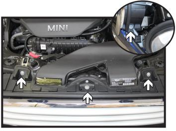
Using a T30 Torx, remove the three (3) screws from the top edge of the fascia.
