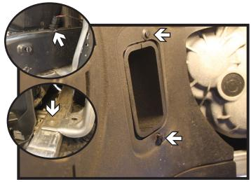
8. In the wheel well, remove the two (2) push pins from the backside of the duct. Remove the duct from the vehicle.
