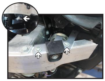
14. Leaving the lower horn loose, reinstall the bracket to the vehicle. After the bracket is reinstalled reattach the lower horn to the bracket.
