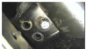
Hold baseplate into opening for tow hook to align with back hole. Insert a 1/2"-13 x 1-3/4" bolt with a 1/2" lock washer and tighten. Refer to baseplate drawing.
