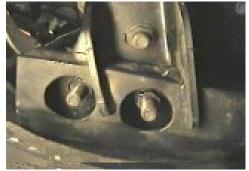
Using a 21MM socket, remove three (3) bolts from each side of the cross member. Set cross member aside to be reinstalled later
