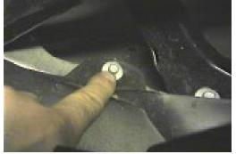
**2.** Using a 6MM socket, remove the nine (9) bolts from the plastic air dam, just under metal bumper.
