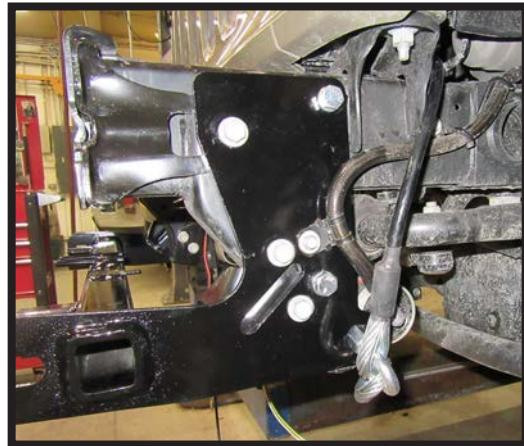
10. **All Models:** Using a 1/2" drill bit, drill the top back hole using the baseplate as a guide. Install the one (1) 1/2" bolt with hardware. Do this on both sides of the vehicle.
