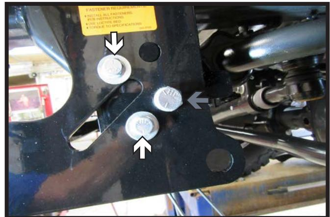
**9b. All Other Models:** Place the spacer plate between the frame and the baseplate. May need to use a pry bar to allow more room for the spacer plate to slide into place. Install the two (2) 3/8" bolts with hardware (white). Then install the one (1) 1 1/2" bolt with hardware into the bottom back hole. May need to ream out the bottom back hole. Do this on both sides of the vehicle.
