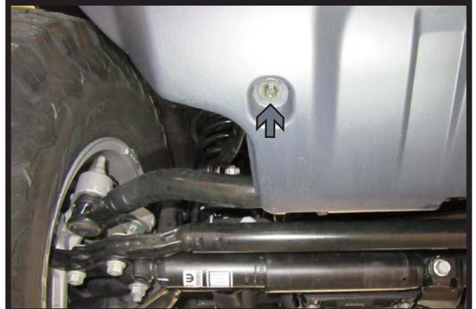
2d. **Overland Models:** Remove the nine (9) push pins from the front edge of the belly pan, there is one (1) in each corner and seven (7) along the center (white). Then using an 8MM socket, remove the two (2) bolts (gray), one (1) on each side, from the belly pan. Remove belly pan and set aside to be reinstalled later.
