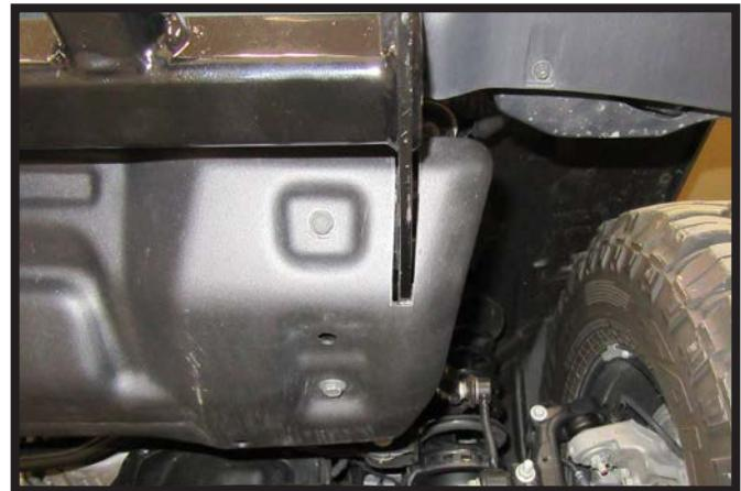
12. Trim belly pan for baseplate clearance in one of two ways listed below then reinstall belly pan.
