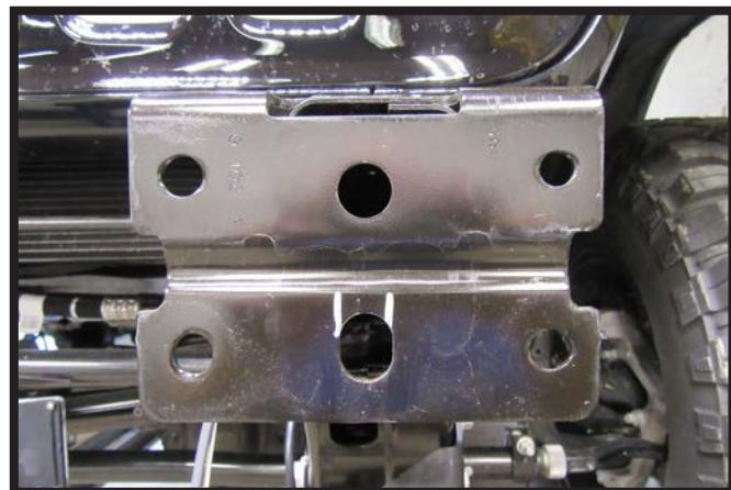
7. Slot the middle bottom hole on the frame as indicated and bend inward to create an access hole. Do this on both sides of the vehicle.
