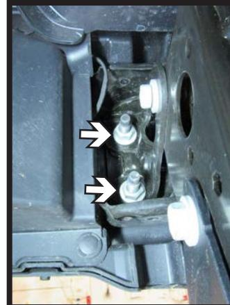
5. Using an 18MM socket, remove the four (4) nuts holding the bumper to the frame. Do this on both sides of the vehicle. Remove the bumper and set aside to be reinstalled later.
