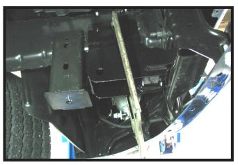
Tip the baseplate at an angle, then slide it into the opening and up to the frame.
