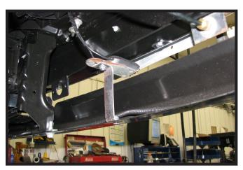
13. Reinstall the lower plastic bumper. There are three holes in the plastic where the breakaway bracket can be attached using a 1/4"-20 x 3/4" bolt with a 1/4"-20 nut. Attach the breakaway to the top of the bracket also with a 1/4"-20 x 3/4" bolt and a 1/4"-20 nut.
