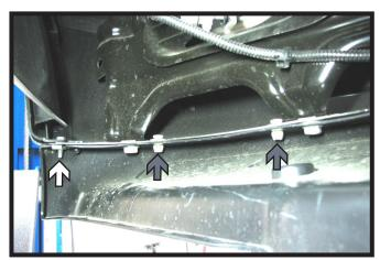
3. To remove the lower air dam, use a 10MM socket and remove the two (2) bolts in each corner of the air dam (white). Remove the thirteen (13) push pins along the seam (gray).
