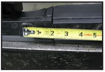
14. On the lower air dam, measure 2" out from the second hole and cut apart. Do this on both sides. Reattach the lower air dam, the plastic bumper and reconnect the plug. If your vehicle is equipped with tow hooks, you will not need to trim the air dam.
