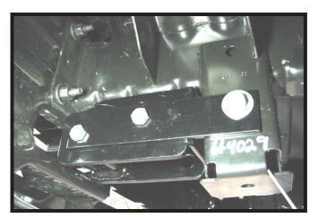
7. On the outer side of the frame install the side mount plate with a 1/2"-13 x 1-1/2" bolt in the front hole, a 1/2"-13 x 1-1/2" bolt and 1/2" lock nut in the middle hole and a 1/2"-13 x 1-1/2" bolt and 1/2" nut wire in the rear hole. Tighten down the bolts and remove the clamp. DO NOT Loctite® the threads, this is a dryfit until all drilling is done. Repeat on the other side of the vehicle.
