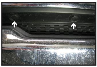
1. **2009-12 Models:** Remove the six (6) push pins along the front plastic insert and remove from the vehicle.
