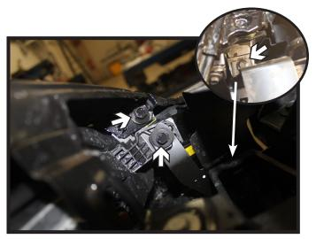
Using a 10MM socket, remove the three
