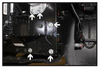
Using a 15MM socket, remove the three (3) bolts from the frame extension and two (2) bolts from the bottom side of the bumper (white). Using a 10MM socket, remove the nut from the fascia extension (gray). Do this on both sides of the vehicle. The extensions will not be reinstalled.
