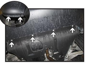
Remove the four (4) rivets from the underside corners of the fascia (inset). There are two (2) on each side. Using a 10MM socket, remove the four (4) screws from the middle portion of the fascia.
