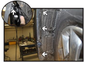
Using a 8MM socket, remove the three (3) screws from the edge of the wheel well. Using a 7MM socket, remove the one (1) screw at the fascia/trim joint (gray). Using a 10MM socket, remove the screw behind the trim (inset). Do this on both sides of the vehicle.
