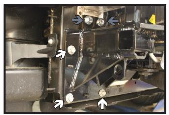
Install the baseplate to the vehicle using the three (3) existing extension bolts (white). Install 10MM-1.25 x 40MM bolts with 3/8" flat washers and 10MM lock washers into the lower bumper bolts (gray). Snug all fasteners, do not fully tighten. Do this on both sides of the vehicle.
