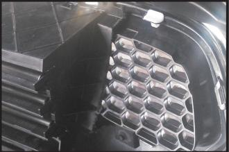
12. **Shutter Models:** The plastic surrounding the outer grille areas must be trimmed to expose the grill behind. Follow the protrusion straight down leaving the areas next to the screws intact. Do this on both sides of the fascia.
