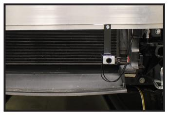
Optional: If installing a breakaway, drill a 1/4" hole thru the bumper lip in the desired location of the breakaway. Attach the bracket to the bumper with the 1/4" x 2" bolt and 1/4" lock nut. Attach the breakaway to the bracket with a 1/4"-20 x 3/4" bolt and 1/4" lock nut.
