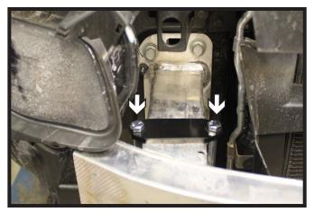
8. Install the support plate and bolts on top of the bumper thru the baseplate. Start the nuts onto the bolts. Fully tighten the frame and bumper bolts in the previous step then the bumper support bolts. Do this on both sides of the vehicle.
