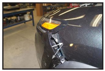
Lift the corners of the fascia up towards the fender (white) and out to release (gray). Continue along under the headlights unsnapping the fascia from the vehicle. Set the fascia aside.
