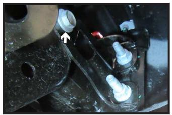
4. Using a 16MM socket, remove the one (1) bolt on the outside of the frame holding the bracket after removing the bumper. Do this on both sides of the vehicle.
