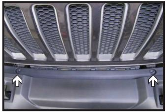
4. Remove the two (2) push pins, directly behind the tow hooks, from the plastic piece between the bumper and the grille. Remove and set aside to be reinstalled later.
