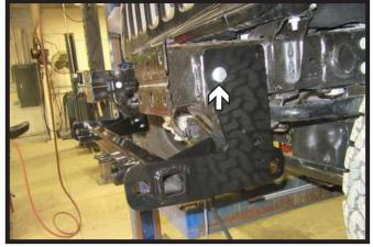
Slide the baseplate onto the vehicle. Start the front 10MM bolt with flat washer and lock washer. Snug bolt up tight so remaining holes line up but do not use Loctite® Red at this time. Do this on both sides of the vehicle.
