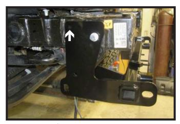
Using a 1/2" drill bit, drill out the top back hole on the outside of the frame using the baseplate as a template. Do this on both sides of the vehicle.
