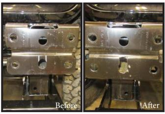
1. Slot the middle bottom hole on the frame as indicated and bend back to create access hole.
