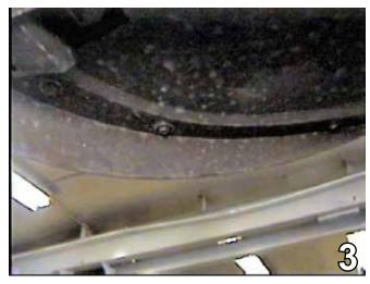
3. Using the 6MM socket, remove three metric bolts, just forward of the front tire. Set metric bolts aside to be reinstalled later. Do this to both sides of the vehicle.
