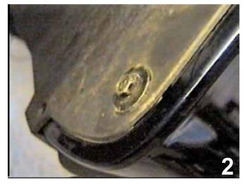
Using the 7MM socket, remove three metric bolts inside the wheel well. Do this to both sides of the vehicle
