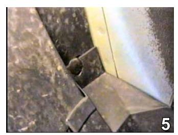
5. Remove one pin tree clip from the upper wheel well. Set pine tree clip aside to be reinstalled later. Do this to both sides of the vehicle.
