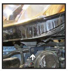
6. Using a 7MM socket, remove the five (5) bolts from the headlight. There are three (3) on top of the headlight area, and two (2) below the headlight on the side. Remove the headlight and set aside. Do this for both sides of the vehicle.
