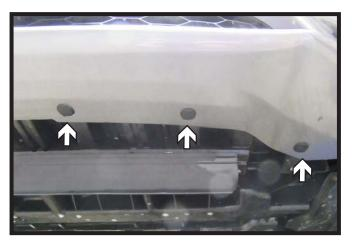
5. Using 10MM socket, underneath the fascia, remove three (3) bolts. Next, remove three (3) push pins. Do this for both sides of the vehicle.
