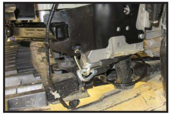
27. Attach the permanent baseplate safety cables to the provided convenience link on the baseplate. The photo above shows the recommended installation of the cables to frame of vehicle. Additional options may interfere with suggested mounting; in this case, secure the cables to a solid piece of the frame as described in the General Information sheet. Be sure the safety cables do not rub against any hoses or moving parts. Do this on **BOTH** sides of the vehicle.
