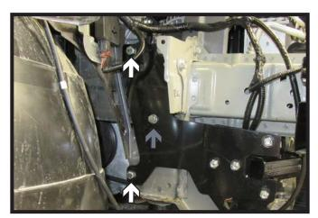
24. On the passenger side insert the two (2) remaining 3/8"-16 x 1-1/4" Hex Head bolts with a flat washer and nylon lock nut on the back as indicated (white). Then insert one (1) 3/8"-16 x 1-1/2" Hex Head bolt and a Whiz nut with 14" wire on the back (gray).
