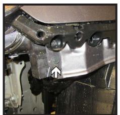
9. Using a 10MM socket, remove four (4) bolts, with two (2) on top, one (1) below, and one (1) on the side. Disconnect the wiring, remove headlights and set aside. Do this for both sides of the vehicle.
