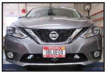
28. Hold the fascia as close to its original position, mark and trim the fascia around the convenience links and attachment tabs. Reinstall the fascia and fascia cover.
