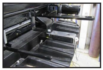
**Optional Breakaway:** Bolt the breakaway to the baseplate bracket with the supplied 1/4" hardware.
