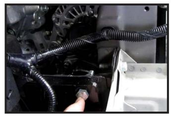
17. Drill one (1) 3/8" hole and start a 3/8" x 2" bolt with a flat washer and nylon lock nut on the back.
