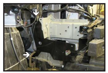
16. Slide on the passenger side plate so that it is level at the top of the frame and flush with the bottom back piece as indicated. Use vice grip to hold into place.
