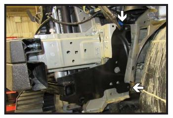
18. Attach cross member so that the driver side plate is level at the top of the frame and flush with the bottom back piece as indicated. Use vise grip to hold into place.
