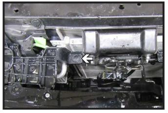
2. Remove the one (1) push pin, and remove the plastic piece.
