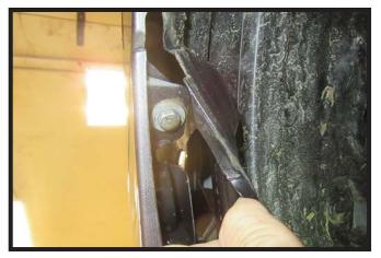
Using a 10MM socket, remove the bolt from behind the wheel well cover where the fascia meets the fender. Do this on both sides of the vehicle.
