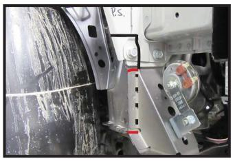
13. On the passenger side use a reciprocating saw to cut along the marked area (black) across and down. Then make two (2) slots (red) as indicated. Using a hammer bend the piece forward along the dotted line.
