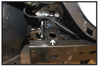
7. Using a 1-1/4" hole saw, enlarge the existing hole on the top side of the frame. Do this on both sides of the vehicle.
