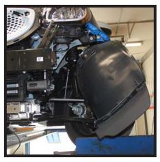
8. Turn the front wheels towards the driver side. In the wheel well, unfasten the plastic screw located along the frame (left). Remove the large push pin located by the fascia/fender joint (middle). Pull the wheel well liner away from the vehicle to access the frame for baseplate installation (right).
