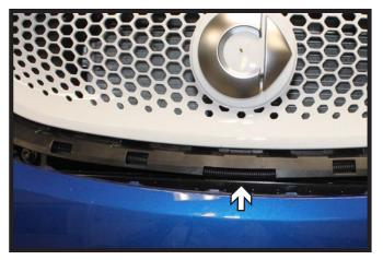
Pull the corners of the fascia away from the vehicle. Disconnect the electrical connection on the passenger side and pull the wire loom out across the front of the vehicle. Set the fascia aside.
