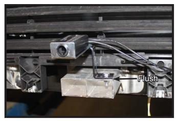
10. Optional Breakaway: Attach the bracket in the desired location flush with the outside of the aluminum tube with the 1/4" hardware. Install the breakaway to the bracket with the supplied 1/4" hardware.
