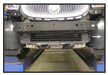
Slide the shroud towards the driver side and remove from the vehicle. The shroud will not be reinstalled.
