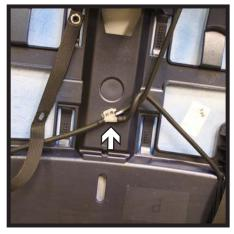
1. Release the hood latch on both sides of the vehicle (left). Pull the hood forward and using a T30 Torx, remove the four (4) screws from the hood straps (middle). Once the hood is free, disconnect the washer fluid lines on the backside at the "Y" section shown (right). Set the hood aside.
