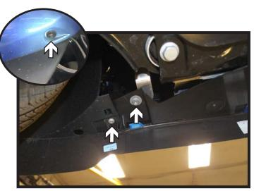
4. Using a T30 Torx, remove the nine (9) screws from the underside of the fascia. There are five (5) in the middle and two (2) on each side.
