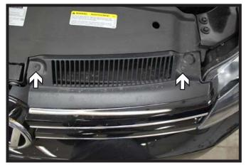
1. Using a T25 Torx, remove the two (2) screws from the top edge of the fascia. There are two (2) on each side.
