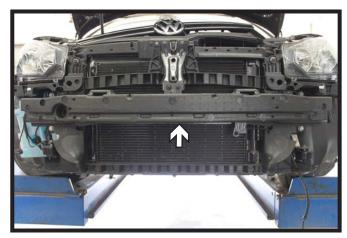
6. Remove the glued styrofoam bumper by prying gently in multiple locations.
