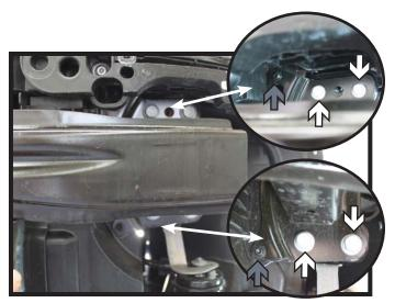
8. On the outer edge of the bumper, using a T30 Torx, remove the two (2) screws (gray). Then using a 16MM socket, remove the four (4) bolts (white). Do this on both sides of the vehicle.
