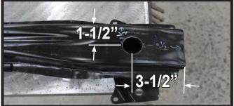
16. On the passenger side, enlarge the hole on the front of the metal bumper just forward of the center of the frame end. Use a reciprocating saw and enlarge the hole or drill out with an 1-1-4" hole saw.
