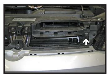
3. Using the T30 Torx, remove the two (2) bolts from the lower grille, one (1) on each side.
