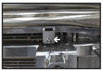
Drill a 1/2" hole in the plate as shown above and insert temperature sensor into hole.
