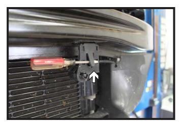
7. Unplug and remove the temperature sensor (white arrow). Take the center piece off for now.
