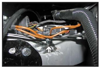
21. On the driver side, drill a 1/4" hole in the edge of the frame. Attach all the ground wires together with a 1/4"-20 x 1" bolt and 1/4"-20 lock nut.
