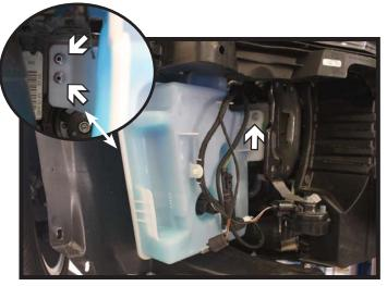
On the passenger side, using a 10MM socket, remove the three (3) nuts from the washer reservoir. There are two (2) on backside and one (1) in front. Disconnect all lines and set the washer reservoir aside.
