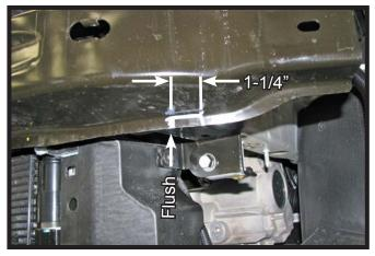
15. **2011-12 Models:** Mark the lower lip of the bumper flush with the outside of the frame rail and 1-1/4" wide. Remove the section of the bumper lip for baseplate clearance.
