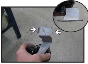
19. Flatten the horn bracket tabs on the passenger side only. Reattach both horn brackets and plug in the electrical connections.
