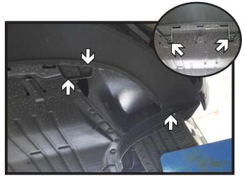
Using a 25 Torx, remove the eight (8) screws from the underside of the fascia. There are three (3) on each corner and two (2) in the center.
