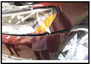
5. Gently, yet firmly, pull outward on the front fascia to remove. Next, remove headlights on **BOTH** sides of the vehicle.
