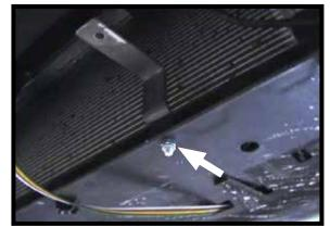
You may place the breakaway bracket anywhere on the vehicle frame. Using a 9/32" drill bit, drill a hole into the frame.
