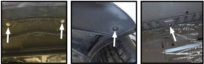
4. On the underside of the front fascia there are seven (7) screws that need to be removed using a Torx 25. There are three (3) on both the driver side and the passenger side, plus one (1) in the center of the vehicle.
