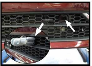
13. Hold the front fascia as close to the original state as possible and mark where the cutout for the convenience links, attachment tabs and breakaway switch, is so equipped, will be located.
