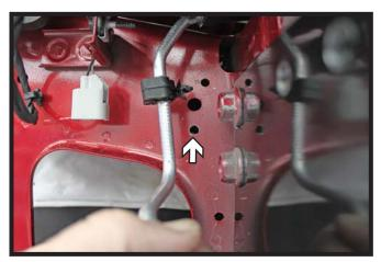
20. On the passenger side, relocate the coolant line to a position that it avoids contact with the baseplate by drilling a new 1/4" hole into the frame face.
