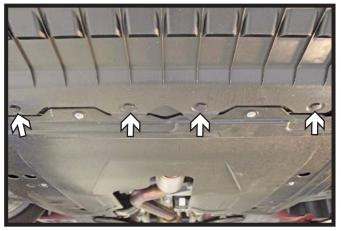
4. Remove the four (4) push pins towards the middle of the underside of the fascia.
