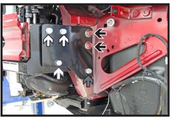
19. One at a time remove the existing frame bolts, apply Loctite<sup>®</sup> Red and reinstall (black). Do this on both sides of the vehicle.
