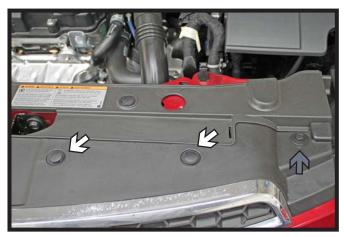
1. Using a 10MM socket, remove the screw from the corner of the fascia (gray). Then remove the two (2) push pins (white). Do this on both sides of the vehicle.
