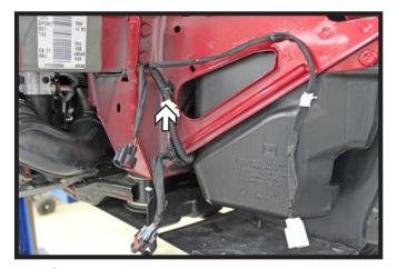
11. On the driver side, remove the wire loom from the frame and move it out of the way for baseplate installation.
