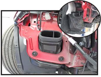
On the passenger side, push back the lower baffle and slide it down to remove it from the vehicle.
