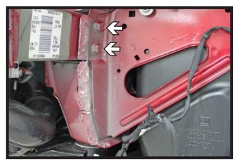
15. Bend the two tabs over and flatten back to the face of the frame. Do this on both sides of the vehicle.
