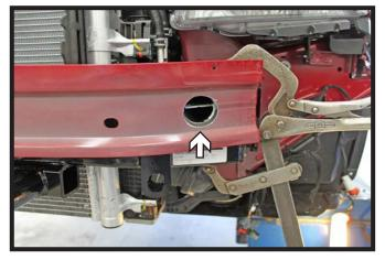
16. Using a 1-1/4" hole saw, drill a hole thru the two layers in the face of the bumper as shown for nut plate access. Do this on both sides of the vehicle.
