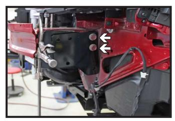
17. Position the baseplate onto the vehicle and temporarily clamp in place. Install the support plates on both sides of the vehicle with the existing hardware and temporarily tighten.
