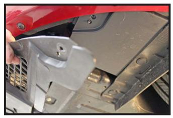
In front of the front tire, pull the lower air dam off the pin. Then pull the lower shield off the pin also in order to remove the fascia.
