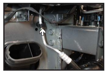
On the passenger side, disconnect the AC coolant line from the holder.
