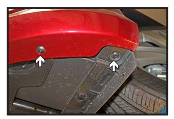
3. Using a T20 torx, remove the two (2) screws from the underside of the fascia. Do this on both sides of the vehicle.
