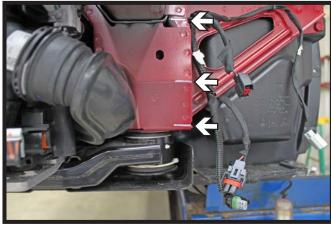
14. Make three (3) slits in the frame face back to the frame side. One just below the upper flange (top). One at the bend in the middle (middle) and one just above the lower bend (lower). Do this on both sides of the vehicle.
