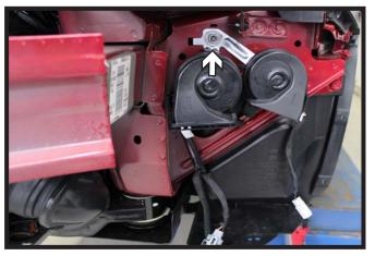
10. On the driver side, using a 13MM socket, remove the bolt from the horn bracket. Unplug and set the horn aside.
