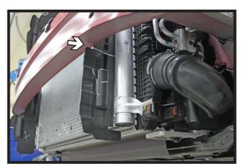
13. Trim the plastic shielding flush with the bottom side of the bumper. Do this on both sides of the vehicle.
