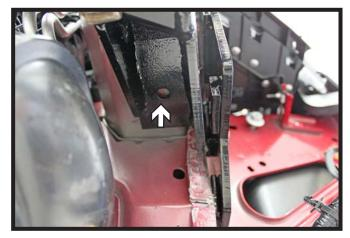
18. Using a 3/8" drill bit, drill the bottom hole thru the frame. Install a 3/8" x 1-1/2" bolt and lock washer into the hole with a 3/8" nut plate on the inside of the bumper. Do this on both sides of the vehicle. Fully tighten all hardware.
